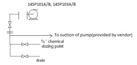
• Following piece to be fitted SBD steam/nitrogen line(water+ chemical injection)
