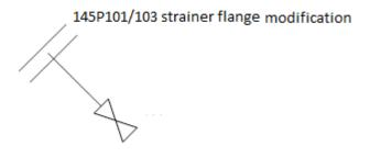
• Drop NRV on LP steam line to column (145C101) and connect the following spool piece.
